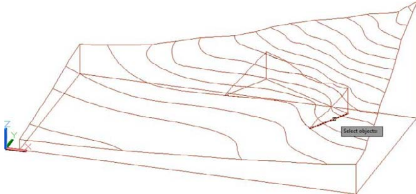
FIGURE 22.57 The 3D solid representing the excavation
